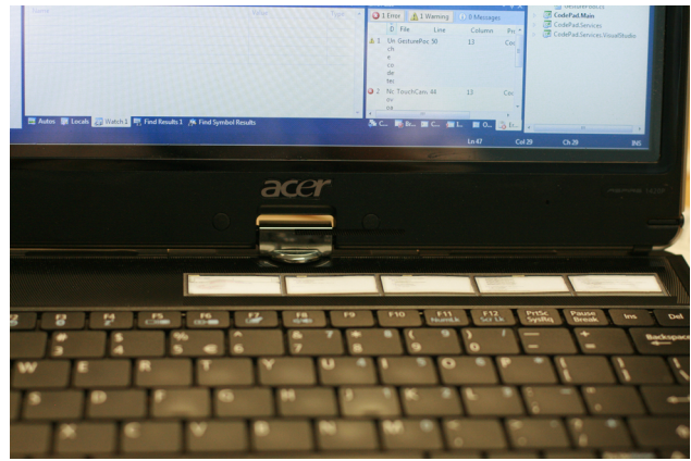
Figure 2: A design suggestion showing how a thin CodePad strip could be integrated with a laptop computer (touchable code documents thumbnails are shown).
